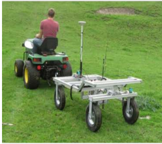
Figure: Detection of soil profiles on pastures; sensor carriage (on the left), detected soil profile
